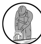
Wear suitable protective clothing with chain saw protected inlays during work.
