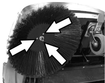
→ Unscrew 3 screws from the underside of the side brush.
