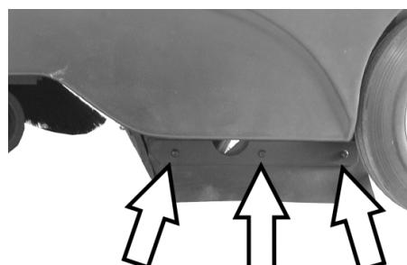
→ Loosen the fastening screws of the sealing strip.
