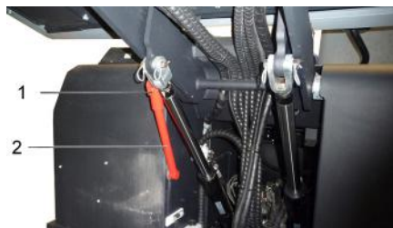
1 Holder of safety rod 2 Safety rod
