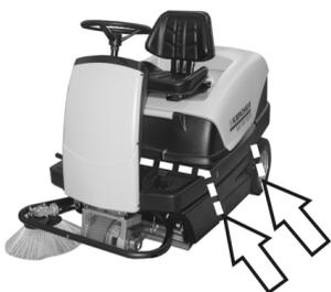
**Note:** Observe markings for fixing points on base frame (chain symbols). When loading or unloading the machine, it may only be operated on gradients of max. 18%.
