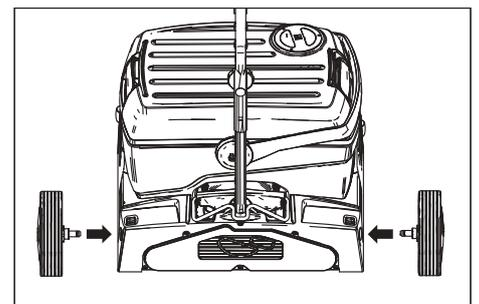
→ Insert the transport wheel axles into the borings on the appliance and lock them.
